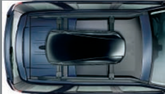
Luggage Box* VPLVR0062 Gloss Black Finish. Opens from both sides. Lockable for security. External dimensions: 1,750mm long, 820mm wide, 450mm high. Volume 440 litres. Load capacity 75kg**.
