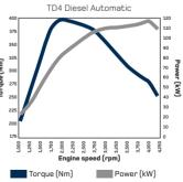
Max torque (Nm) Max power (kW) 400Nm/2,000rpm 118kW (160PS)/4,000rpm
