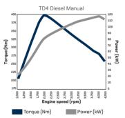
Max torque (Nm) Max power (kW) 400Nm/2,000rpm 118kW (160PS)/4,000rpm
