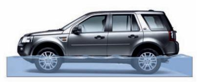
Wading Depth Maximum wading depth 500mm
