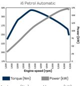
Max torque (Nm) Max power (kW) 317Nm/3,200rpm 171kW (233PS)/6,300rpm
