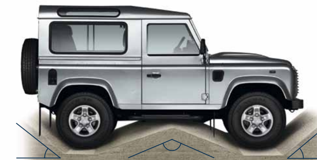
Departure angle Ramp angle Approach angle
