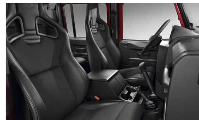
Recaro Front Seat Kit** VPLDS0036PUY – Left-hand seat VPLDS0035PUY – Right-hand seat Heated seat with cloth seat facings and leather surround, featuring Land Rover and Recaro embossed logos. Installation kit included. Not compatible with vehicles fitted with a bulkhead or 90 bulkhead deleted vehicles with jack stowage brackets behind the front seats. Applicable VIN WA138480 110SW, 110 and 130 Double Cab and 9A773310 90 vehicles with bulkhead deleted. Compatible with vehicles fitted with heated seat option. Supplied individually.
