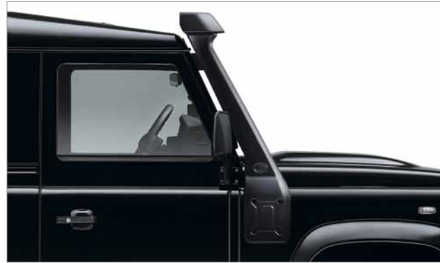
Raised Air Intake LR008383
