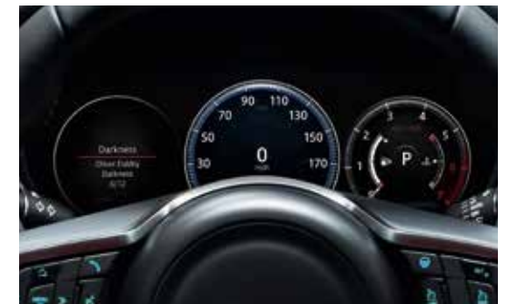
12.3" Full Digital Instrument Panel with virtual dials
