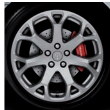
Light alloy wheels - 7-spokes "V" Style (8.5J x 19" front; 10.5J x 19" rear) Standard on Quattroporte S
