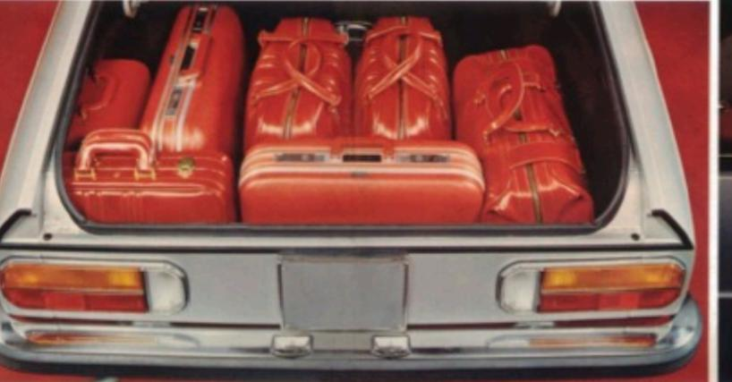
The boot is exceptionally big for a sporting coupé. Like the engine compartment it is lit internally, on opening, from the side light circuit. The covered spare wheel is instantly accessible.
