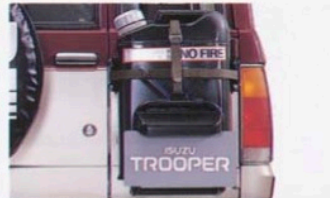
Spare fuel tank
