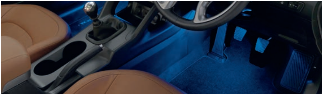
Blue LED lighting foot area Concealed floor illumination for the front foot space. It provides welcome illumination that automatically switches on and off with the opening and closing of the front doors. Part Number: 99650ADE00
