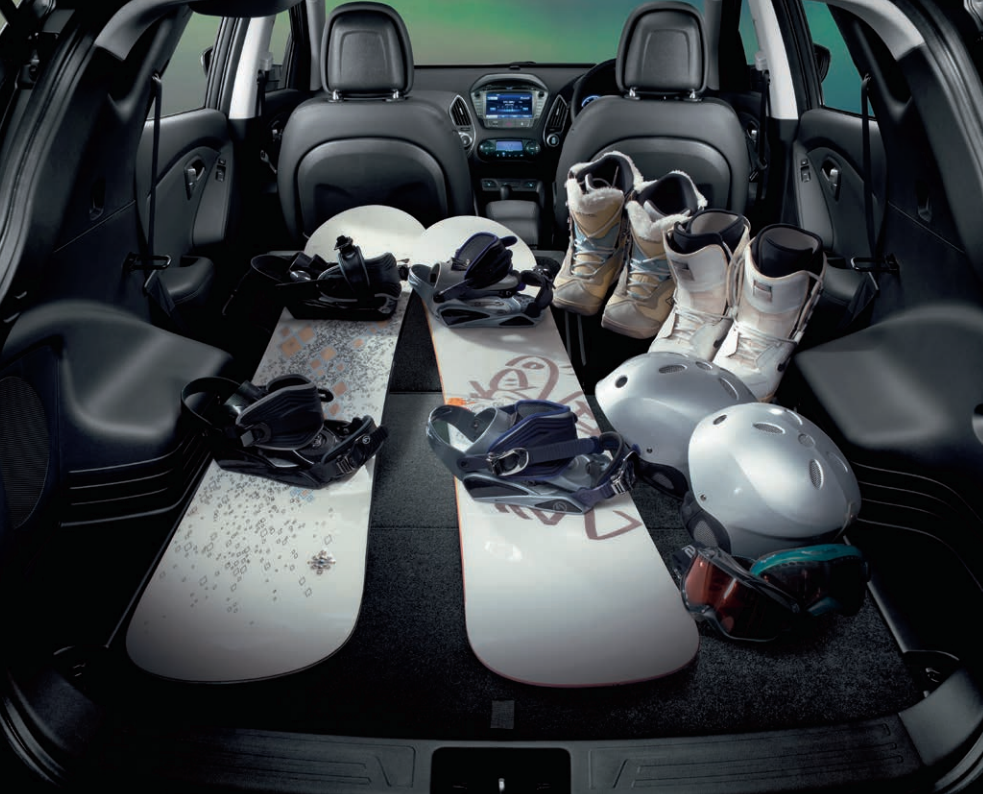
Split-fold rear seats. The rear seats are individually foldable so you can carry one or two rear seat passengers and still accommodate lengthy cargoes.
