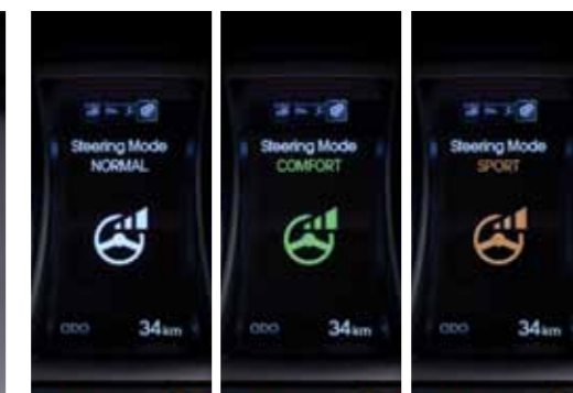
With optional Flex Steer you can adjust the steering performance to your personal driving style: it includes Comfort mode for easy parking and urban driving, Normal mode, and Sports mode for motorway driving.
