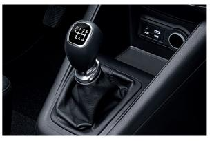
**Six-speed transmissions.** Diesel engines have 6-speed manual transmissions, as does the 1.6 petrol engine, which can also be specified with a new, high-efficiency 6-speed automatic transmission.
