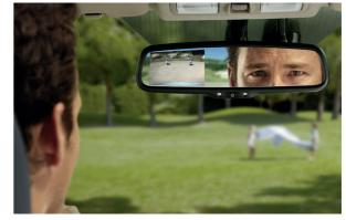
**Rear parking assist.** Reversing into confined spaces is simplified by parking sensors providing audible warnings of obstacles, and a rear camera that is monitored via the navigation screen or rear-view mirror.
