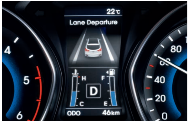
Lane Departure Warning System. Instant visual and audible warning of unintentional departure from the lane you're driving in.
