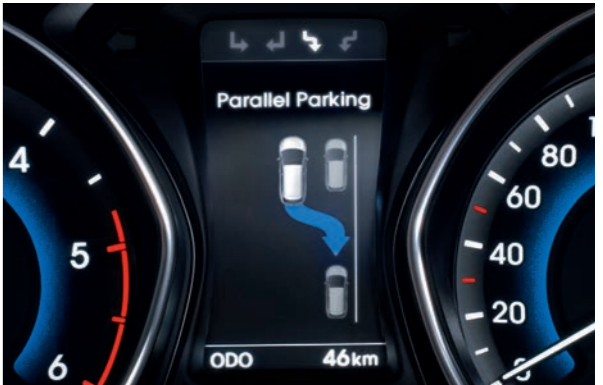
Smart Parking Assist System (SPAS). Activated sensors can identify a viable parking space, then steer the i30 perfectly into the available space. You control the accelerator and brake, the system does the rest.
