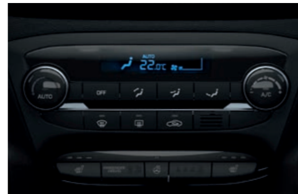
Automatic climate control. Select your preferred temperature and the system does the rest. Its auto-defog function keeps the windscreen clear.
