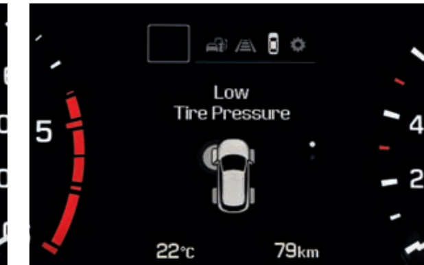
Tyre Pressure Monitoring System. Senses and indicates the loss of pressure in individual tyres.
