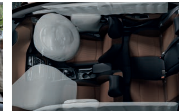
6 airbags. All-round protection with 2 front, 2 side and 2 curtain airbags.
