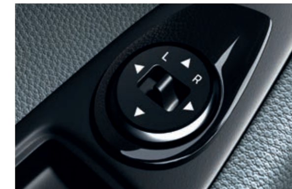
Powered and heated door mirrors. The door mirrors can be remotely adjusted and heated from the door console.
