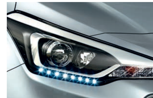
High performance projector headlamps. Combined with LED daytime running lights.
