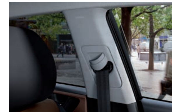
Height-adjustable seat belts. The upper front seatbelt mounts are height-adjustable for improved safety and comfort.
