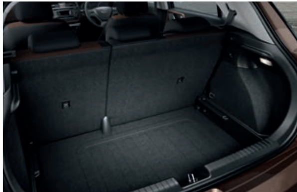
Adjustable load space floor. The luggage floor can be located at 2 different heights to create either a flat load floor when seats are folded flat, or a deeper load space if preferred.
