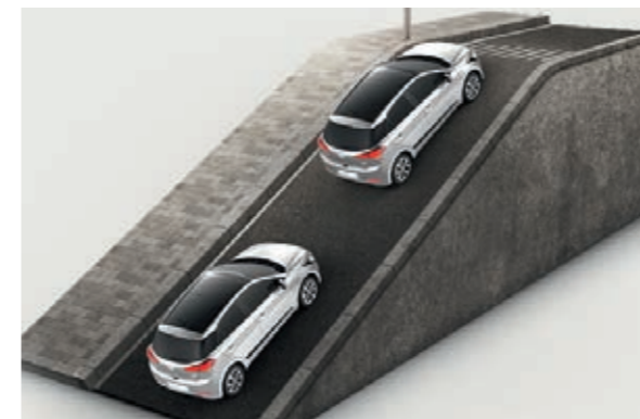
Hill Start Assist Control. Prevents unintentional rollback when starting on hills.
