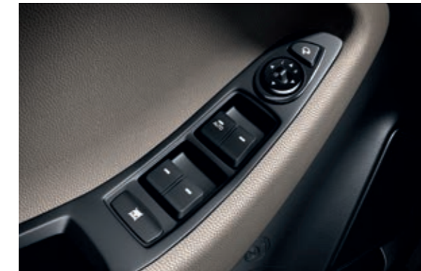
Electric windows, front & rear. All side windows can be raised and lowered remotely. Front windows have a one-touch Auto up/down function.
