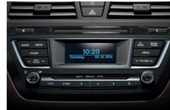
Audio system. RDS radio with CD/MP3 player and Bluetooth connectivity and 1GB storage. The system can also be operated by controls on the steering wheel (deluxe model upwards). The Bluetooth brand is the property of Bluetooth SIG Inc
