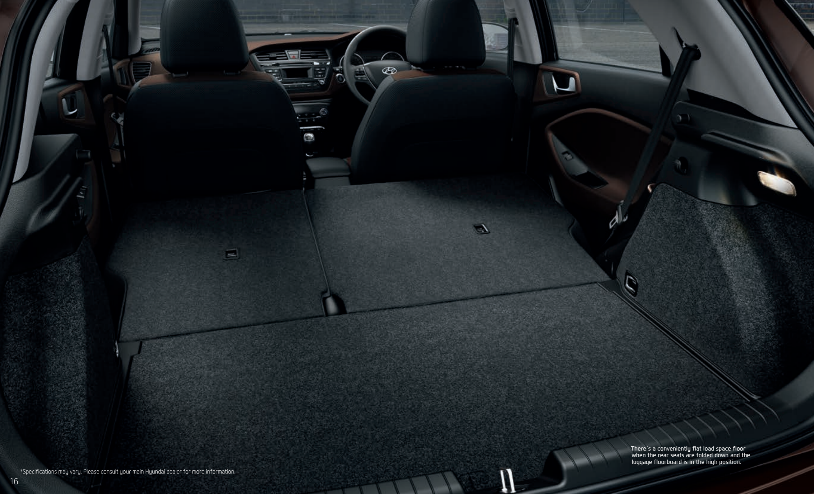
Split-fold rear seat. The rear seats can be folded flat in the ratio 60:40 to create a conveniently versatile load space.
