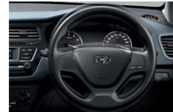
Adjustable steering wheel. The steering wheel is adjustable for both reach and rake.
