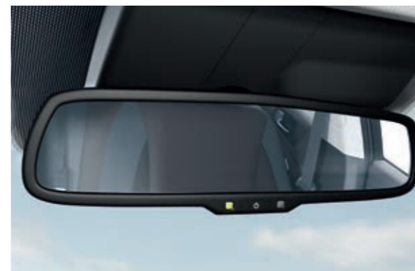
Electro-chromatic mirror (ECM). The interior mirror automatically darkens when its sensor detects glare from the headlights of following vehicles.
