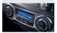
Full auto air conditioning GL and GLS trim can be ordered with fully automatic air conditioning which includes a digital readout. Just pre-set the desired temperature and it will be automatically maintained.
