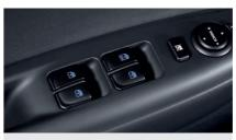
Multi control switch Adjustment of the side view mirrors and power window switches are accessible from this conveniently located control module.
