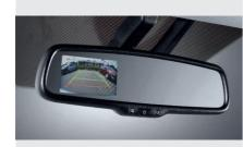
ECM mirror with rear view camera display The electro-chromic mirror self-adjusts reflectivity between day and night driving and is available on all trims.
