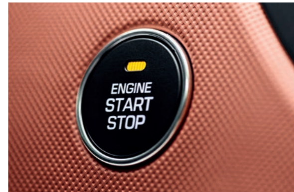
Engine start/stop button. Keyless starting when the smart key is on board in your pocket or bag.
