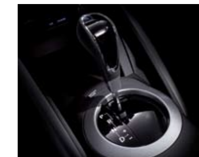
Automatic transmission The 6-speed automatic transmission features fully variable line pressure control and oil pressure deviation adjustment.
