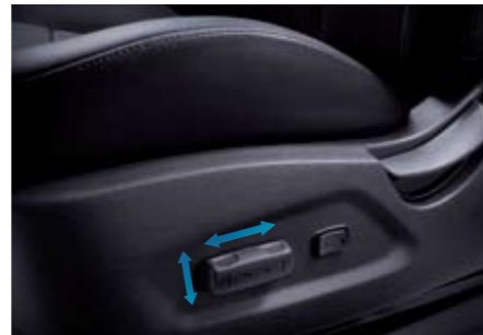
4-way power seat A power seat function allows the front seats to be adjusted at the touch of a button. Provides forward / back as well as cushion height adjustment.
