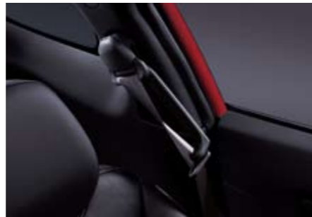
Seatbelt extension guide A seatbelt extension guide for the driver seat puts the belt in the optimum position for comfort and convenience.
