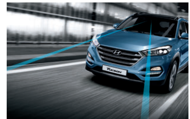
Lane Keeping Assist. Instant visual and acoustic warning, plus corrective steering intervention, when unintentional lane departure is detected.
