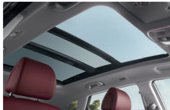
Panorama sunroof. The extra-large panorama sunroof adds the feel of open-air driving. At the touch of a button you can fill the interior with fresh air and sunlight. An automatic wind deflector minimizes noise and buffeting.
