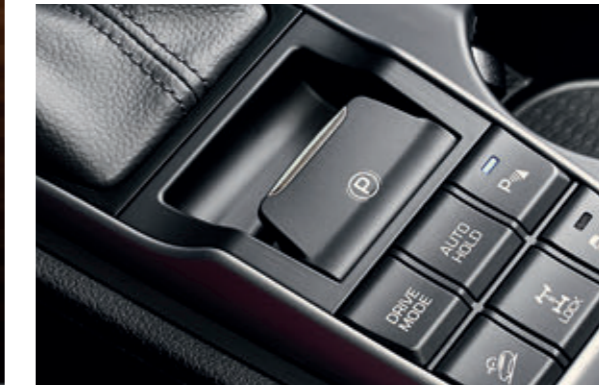
Electronic parking brake. The compact parking brake control frees up useful interior space between the front seats, and is convenient due to the auto brake release function.
