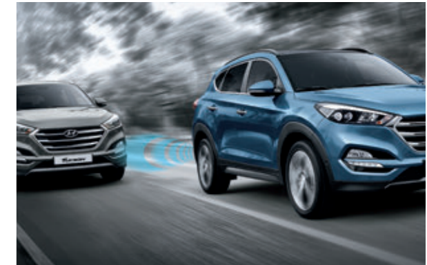
Blind Spot Detection (BSD). Sensors mounted in the car's rear flanks detect the proximity of any vehicle obscured in the blind spot, and trigger an acoustic warning if a turn signal is activated.
