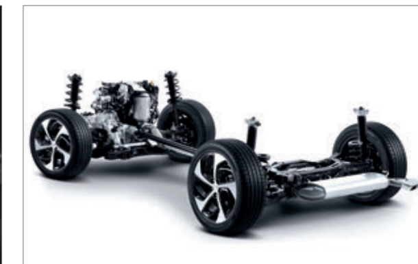
On-demand 4WD. When a potential loss of traction is detected, up to 50% of torque is transferred to the rear wheels for improved grip on loose, slippery surfaces and enhanced cornering performance. Torque distribution can be locked in 50:50 mode in extreme conditions.
