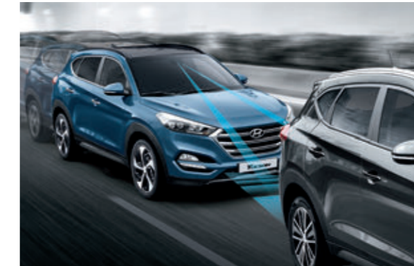
Autonomous Emergency Braking (AEB). The radar and camera based Front Collision Warning System (FCWS) alerts the driver of potentially dangerous proximity of vehicles and pedestrians and brakes autonomously if required.
