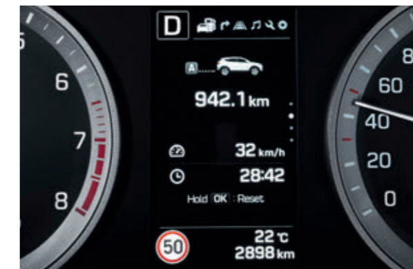
Speed Limit Information Function (SLIF). The system recognises road-side signs, cross-checks with navigation data and displays the current speed limit in the navigation screen and the high-resolution TFT display.
