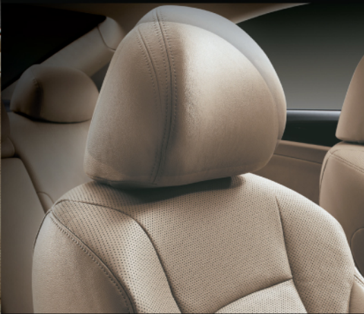
ACTIVE HEADREST In the event of a rear-end collision, active headrests channel the force of the driver and passenger's size and weight to help support the body.
