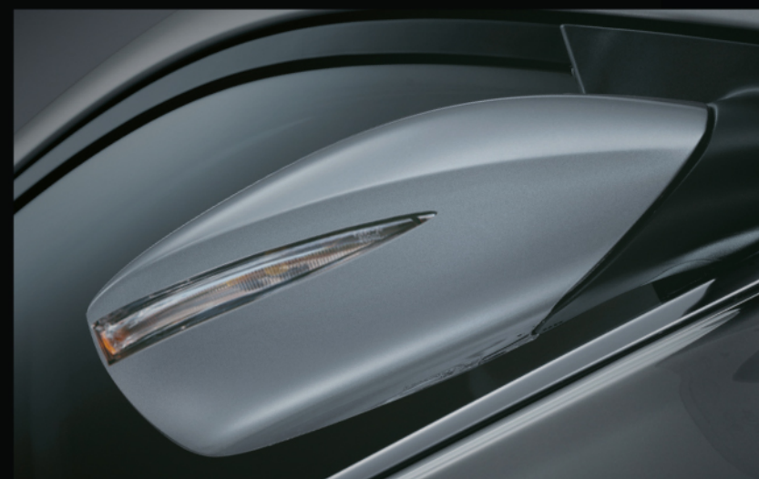
LED OUTSIDE MIRROR SIDE REPEATERS Seamlessly encased into the surface of the housing, the LED lamps on the wing mirrors offer enhanced visibility to oncoming traffic while cornering.
