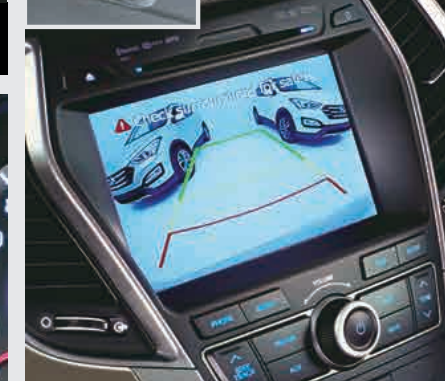
Rear Parking System: A rear-view camera with a display on the touch audio screen and rear parking sensors promotes safer parking.
