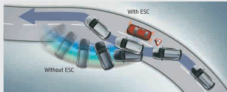
ESC (Electronic Stability Control/4WD Assistance Control): Technologically advanced ESC ensures optimal braking performance by automatically delivering the right amount of braking force to each wheel based on engine torque and driving circumstances.
