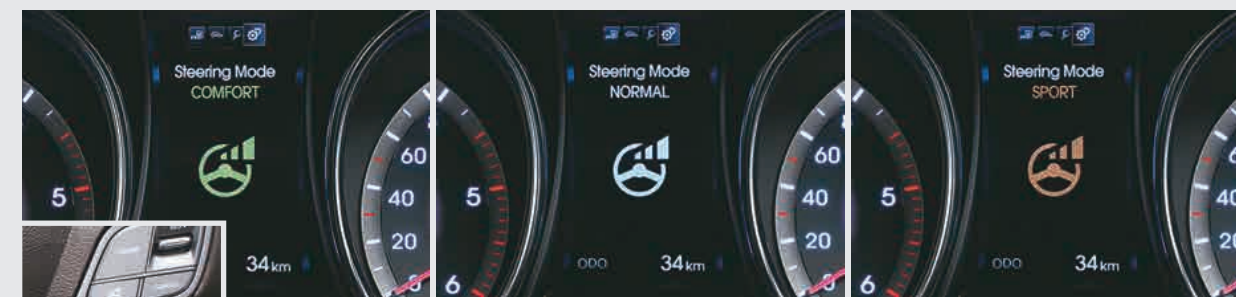
Flex steer™: Flex Steer enables drivers to choose among three driving modes (Normal/Sport/Comfort) according to their preference. The dedicated switch embedded in the steering wheel is easy to operate and can be switched on while driving.
