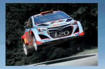
The hand-built i20 WRC is a high-performance competition car based on the popular production vehicle. Developing more than 300 PS of power and 400 Nm of torque from a 1.6-litre engine and weighing 1,200 kgs, it requires highly-skilled drivers and co-drivers to handle its immense power.
