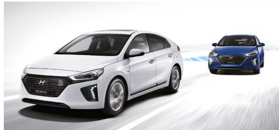
Blind Spot Detection (BSD): rear radar sensors detect the proximity of other vehicles when changing lanes or backing out of parking spaces.
