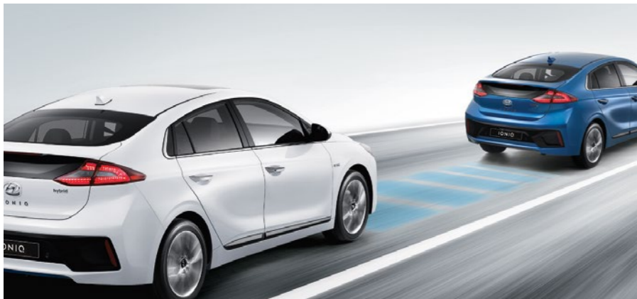
Smart Cruise Control (SCC): maintains a safe distance between you and the preceding vehicle.
