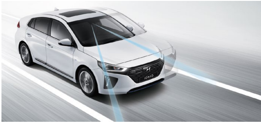
Lane Keeping Assist System (LKAS): warns the driver of unintended departure from the chosen traffic lane and applies corrective steering if necessary.
