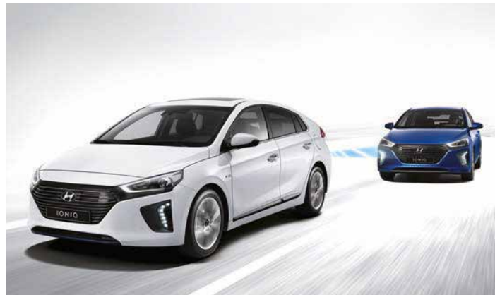
Blind Spot Detection (BSD): rear radar sensors detect the proximity of other vehicles when changing lanes or backing out of parking spaces.
