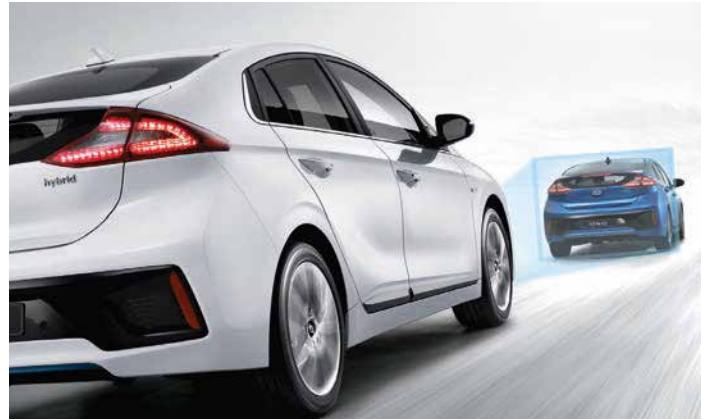
Autonomous Emergency Braking (AEB): when a potential collision with a vehicle or pedestrian is detected, AEB first gives a visual and an audible warning, then intervenes with partial or complete brake application.
