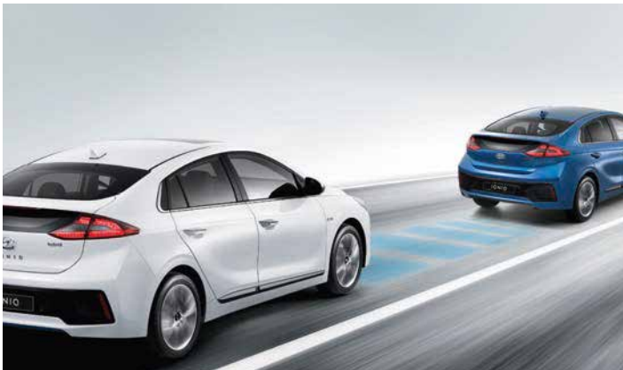
Smart Cruise Control (SCC): maintains a safe distance to the preceding vehicle.
