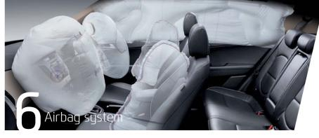
The latest depowered-type front airbags serve the driver and front seat passenger. Side airbags protect the thorax and pelvic areas of the driver and front seat passenger. Curtain airbags provide head protection across the side window areas.
