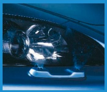
To ensure that the triple beam projector headlamps maintain their efficiency, powerful headlight washers are fitted as standard.
