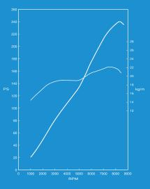
The Honda DOHC VTEC engine combines low rev torque with high end power
