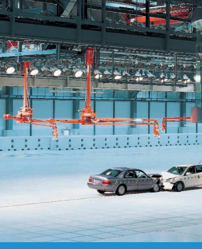
The Honda S2000 has been subjected to vigorous safety tests. We know just how hard a test regime the car's been through, as we built the test-facility centre ourselves. Our crash test centre in Tochigi, the largest in the world, has allowed us to test impact resilience from all possible directions, just as it can happen in real life. Within the car's frame are built-in crumple zones. These ensure that if an accident happens, the sections deform
