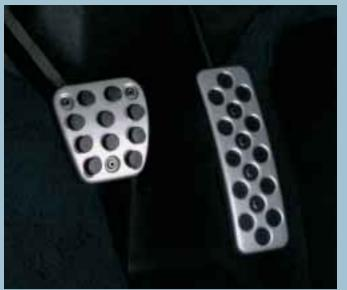
The foot pedals are drilled aluminium alloy making them light and sensitive for instant, precise responses.
