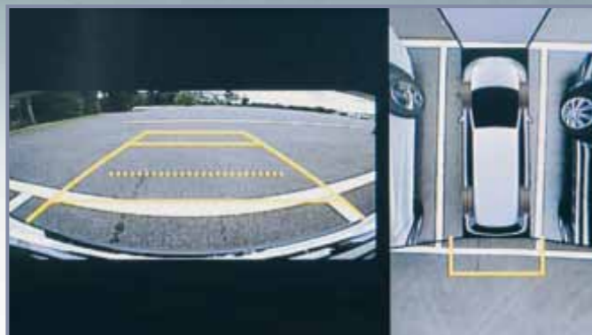
The multi-view camera system offers a composite view of the car's surroundings through multiple wide-angle views on the vehicle's navigation screen.
