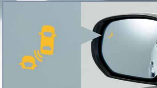
The Blind Spot Information beeps if there's an approaching vehicle, and an indicator light will appear on the side view mirror.
