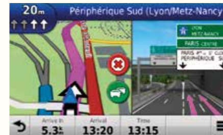
GARMIN NAVIGATION † Garmin PhotoReal™ displays upcoming junctions with photo-realistic images of exits with arrow lane indication to provide clear guidance. The system also includes predictive routes, real-time traffic avoidance, road speed limit display, 3D buildings, terrain views and more.
