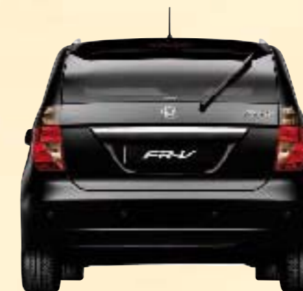
Height 1610mm (1625mm including roof rails, 1770mm including aerial)
