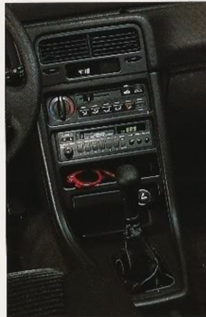
The center console is designed to house the push-button temperature controls, an available AM/FM stereo with cassette and a quartz digital clock, with room left over for cassette tapes and personal items.
