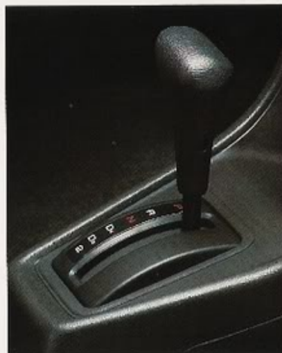
A 4-speed automatic transmission, rarely seen in a car of this class, is available with electronically controlled lockup torque converter.
