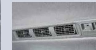
2ND ROW ROOF AC VENT
