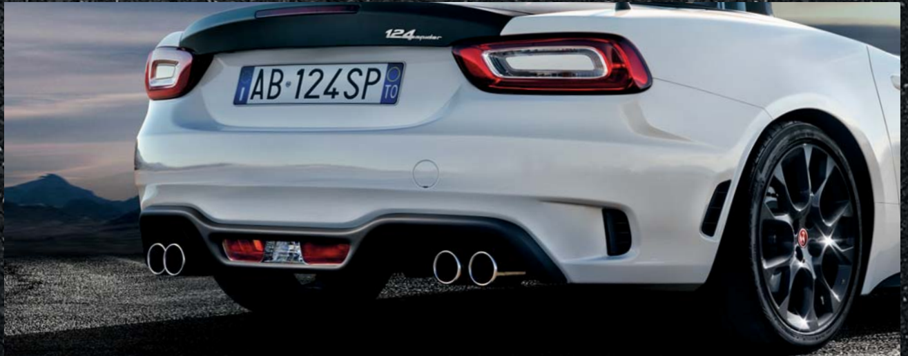
Aerodynamic Diffuser. To increase the road handling.
