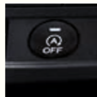
IDLE STOP BUTTON (manual transmission only)
