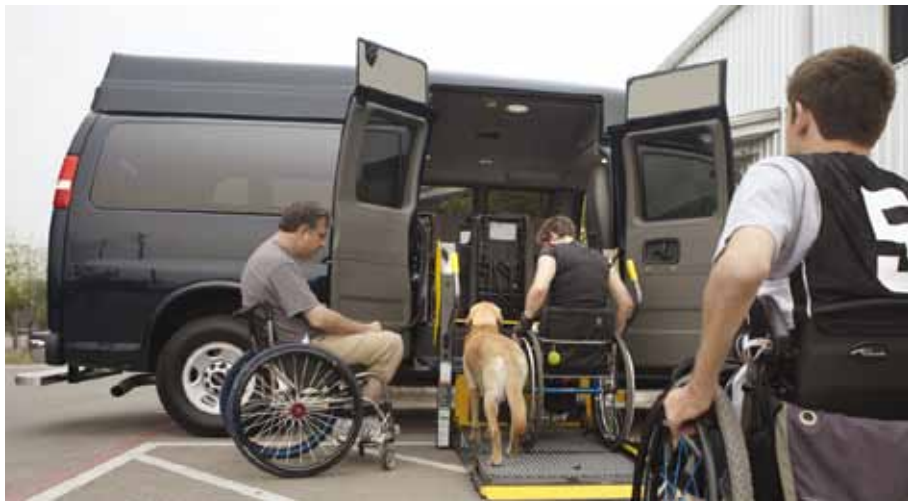
↑ Savana's frame readily accepts a raised roof, wheelchair lift and entry options and retractable wheelchair securement systems for easy mobility conversion.
