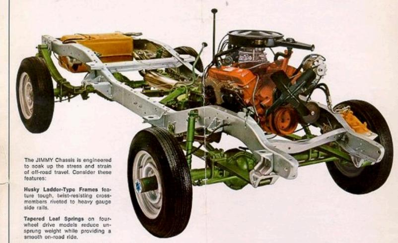
Vari-Rate Rear Springs ride smoothly when lightly loaded, stiffen up for extra support when loaded.
