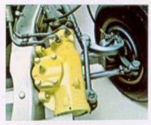
Power Steering. Optional integral-type unit reduces steering effort to combat driver fatigue. Dampens road shock at steering wheel for added comfort.
