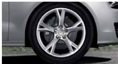
Cast aluminium wheels in 5-arm Y design size 8.5 J x 19 with 255/40 R 19 tyres*
