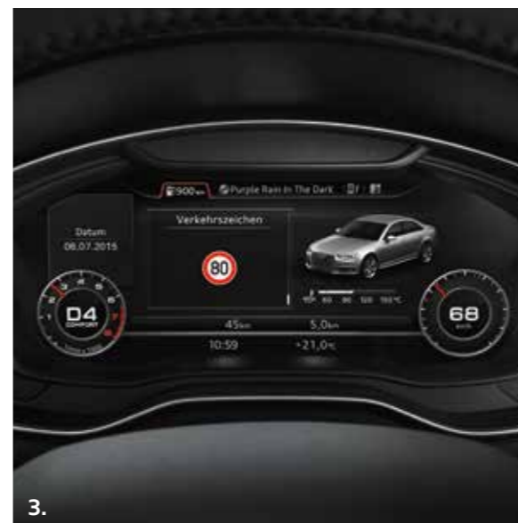
1. Head-up display (KS1). 2. Rear view camera (KA2). 3. Camera based traffic sign recognition (QR9). 4. Advanced key, with electric hands-free boot opening system (PGD or PGB).
