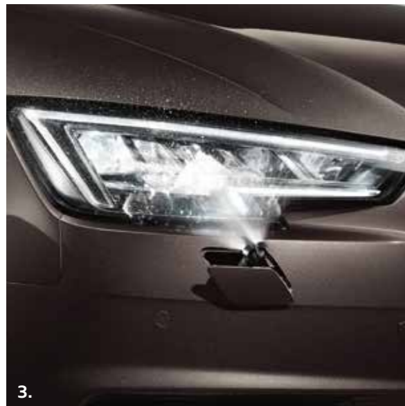
1. Matrix LED headlights with LED rear lights and dynamic front and rear indicators (PXC). 2. Dynamic rear indicators (PXC or PX2). 3. Headlight washers (8X1). 4. LED headlights with LED rear lights and dynamic rear indicators (PX2).
