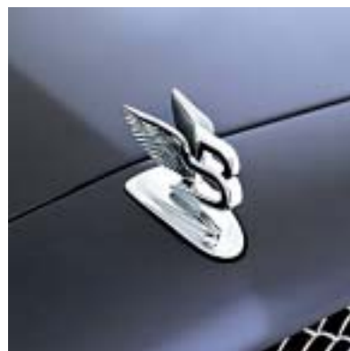
RETRACTABLE FLYING 'B' RADIATOR MASCOT (PAINTED RADIATOR SHELL)
