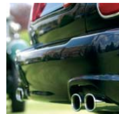
REAR SPORTS BUMPER AND QUAD EXHAUST TAIL PIPE FINISHERS
