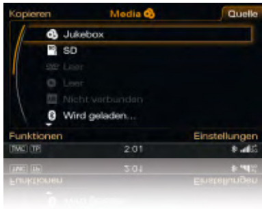
Media: Display of available media sources such as the jukebox, inserted SDHC cards, Audi music interface or CDs and DVDs; display of optional TV tuners.
