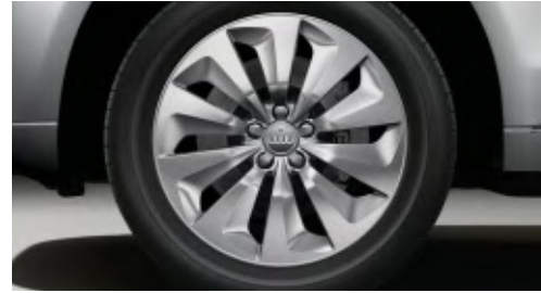
Cast aluminium wheels in 10-arm turbine design (hybrid design) size 8 J x 19 with 235/55 R 19 tyres
