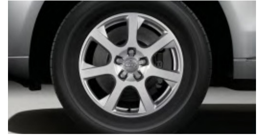
Forged aluminium winter wheels in 7-spoke design 1 size 7 J x 17 with 235/65 R 17 tyres, can be fitted with snow chains, permissible top speed 210 km/h
