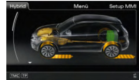
Combined driving in hybrid mode with combustion engine and electric motor
