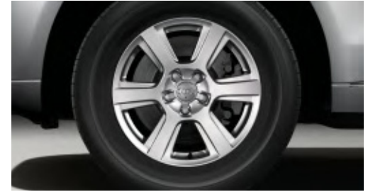
Cast aluminium winter wheels in 6-arm design 2 size 7 J x 17 with 225/65 R 17 tyres, can be fitted with snow chains, permissible top speed 210 km/h
