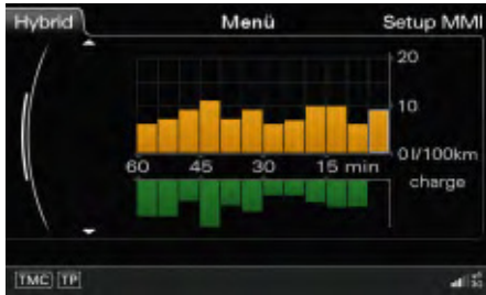
Two bar charts visualise the average consumption of the combustion engine (orange) and the recuperation amount of the electric motor (green) in 5-minute intervals.
