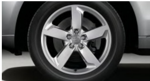
Cast aluminium wheels in 5-arm design partly polished, size 8 J x 19 with 235/55 R 19 tyres
