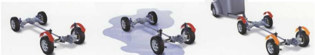
When braking, the car disengages drive to the rear wheels the moment you touch the brake pedal, preparing itself to maximise control and roadholding.
