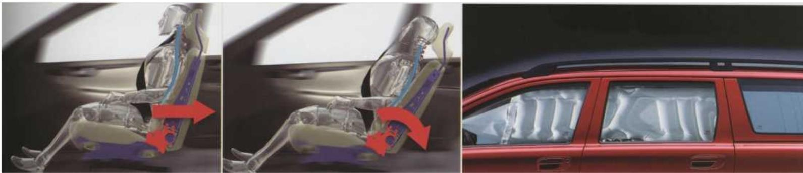
WHIPS (Whiplash Protection System) reduces the strain on the spine and neck in rear-end collisions. It is integrated in the front seats and is activated by a sufficiently severe rear impact.
