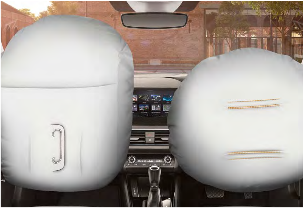
FRONT AIRBAGS While the driver airbag is enclosed in the steering wheel, the passenger airbag is located in the dashboard.
