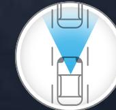
**INTELLIGENT EMERGENCY BRAKING** is your ally in traffic and busy city streets. It monitors your speed and distance between you and the car ahead, and can let you know if you need to slow down. It can even automatically engage the brakes to help avoid a collision or lessen the severity of an impact. And when it detects a pedestrian in the crosswalk, it can apply the brakes for you.
