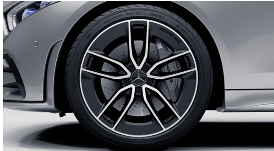
RTZ 20" AMG alloy wheels (4) – 5-twin-spoke design, front: 245/35 tyres, 8J x 20 ET 10 wheels; rear: 275/30 sports tyres, 9J x 20 ET 28 wheels and TIREFIT with tyre inflation compressor
