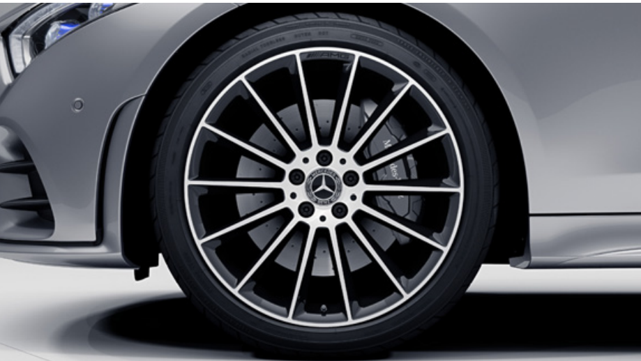
RVP 20" alloy wheels (4) – multi-spoke design, painted in black with a high-shine finish, front: 245/35 tyres, 8J x 19 ET33 wheels; rear: 275/30 run-flat tyres, 9J x 19 ET28 wheels
