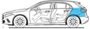
Open luggage compartment behind rear seat, loaded to upper edge of rear seat backrest, volume 310 litres (V 211-2)
