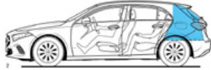
Open luggage compartment behind rear seat, loaded to roof, volume 375 litres (V 214-2)
