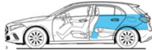
Open luggage compartment behind driver's seat, rear seat backrest folded, loaded to upper edge of driver's backrest, volume 780 litres (V 211-1)
