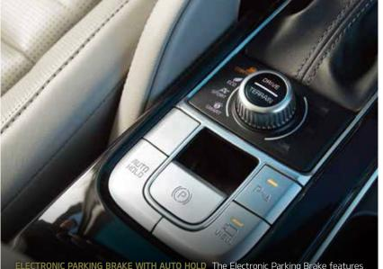
**ELECTRONIC PARKING BRAKE WITH AUTO HOLD** The Electronic Parking Brake features Auto Hold, operated by a button on the center console behind the gear selector. The hold feature is especially useful when waiting on a steep incline. It will prevent the vehicle from rolling back as you wait to proceed.
