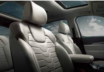
**VENTILATED SEATS** Ventilated front seats use fans, heating elements and small perforations to help the driver and front passenger get and stay comfortable. Ventilated and heated captain's chair seats are also available for the second row, a first among SUVs in this class.
