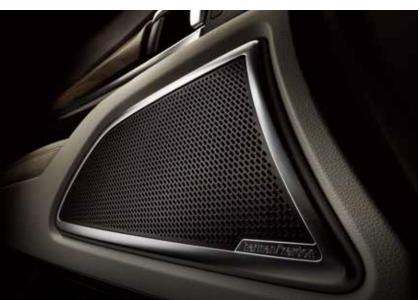
HARMAN KARDON SOUND SYSTEM The Harman Kardon premium sound system transforms a ride in the spacious Telluride cabin into an auditory adventure. Its external amplifier drives 12 precisely positioned speakers, including an OCS-type subwoofer that generates bass output markedly superior to that of a conventional enclosed subwoofer.
