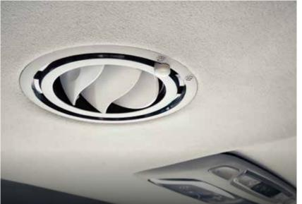
**ROOF-MOUNTED REAR CLIMATE CONTROL AND 360° VENTS** First-in-class roofmounted rear-seat climate controls let people in the second row adjust the temperature, strength, direction, and mode of airflow that reaches them. Diffusible 360° air vents in the roof let rear passengers stop, reduce or redirect airflow.
