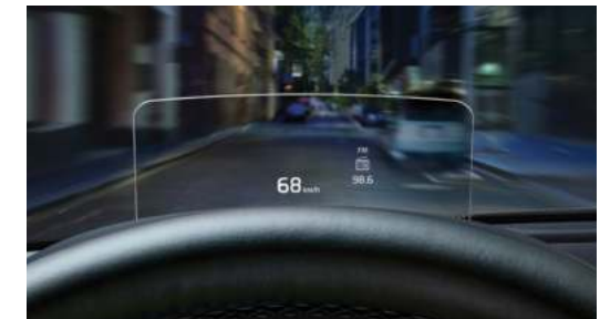
Heads-up display (HUD) 1 subtly projects key driving information on a secondary screen above the steering wheel.
