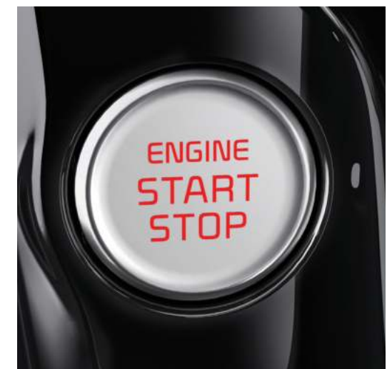
Smart key with push-button start 1 lets you start your vehicle with your key in your pocket.
