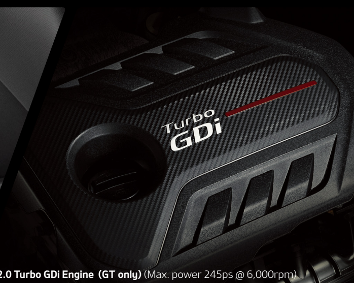
2.0 Turbo GDi Engine (GT only) (Max. power 245ps @ 6,000rpm)
