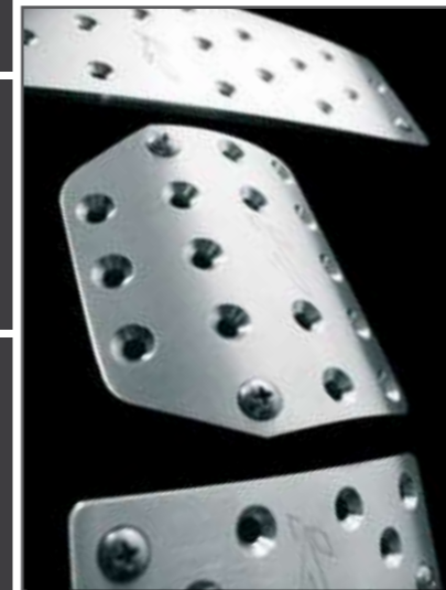
Vented Foot Pedals in Machined Aluminium
