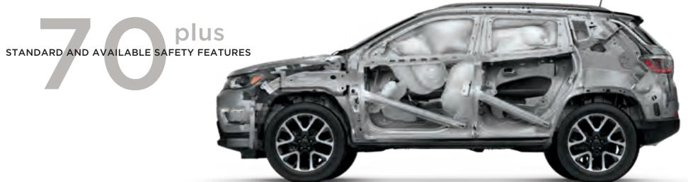
A Secure Air Bag<sup>8</sup> System Your need for security is fully respected with this all-around air bag<sup>8</sup> system. Full-length side-curtain, seat-mounted side thorax, and advanced multistage front and driver's inflatable knee bolster air bags<sup>8</sup> all work together to help provide protection. Standard.
