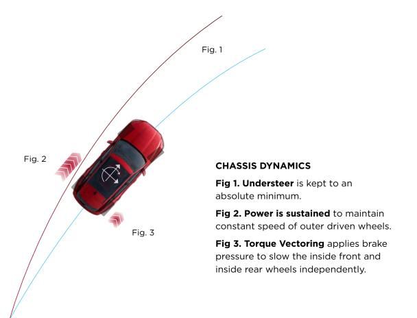
When straight roads become snaking roads, F-PACE's Torque Vectoring by Braking makes all the difference. It provides controlled independent braking on the inside front and rear wheels to maximise capability through even the tightest corners. Together with Dynamic Stability Control, it corrects understeer, giving the vehicle its sports car-like agility and providing you with extra confidence when driving.
