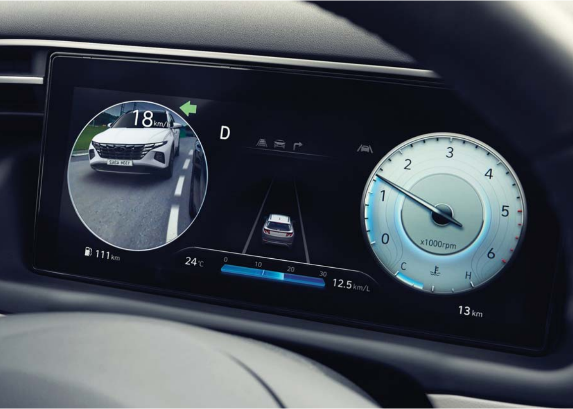
Blind-spot View Monitor When using the turn signal, the camera installed at the base of the exterior mirror displays videos of the left/right posterolateral views on the cluster screen.
