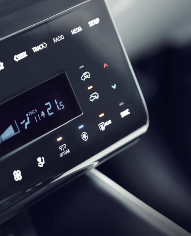
Multi Air Mode / After-Blow automatically dries the air conditioner Touch the Multi Air Mode button ("Diffuser") to summon a subtle breeze that refreshes the air in the cabin. The After-Blow system activates a fan for a pre-determined period of time after the engine is turned off to dry any remaining condensation and reduce unpleasant odors. * After-Blow can be activated via a menu in the infotainment system. * After-Blow is not available on the Hybrid.
